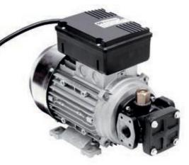
Internal gear electric pumps for lubricants. 230 V - 50 Hz (single-phase) or 380 V - 50 Hz (three-phase) motor, depending on model, IP-55 protection and on/off switch. Cast iron pump body, sintered steel gears and by-pass valve. Motor with mounting feet, the pump can be mounted horizontally on a flat surface or vertically on a wall.
